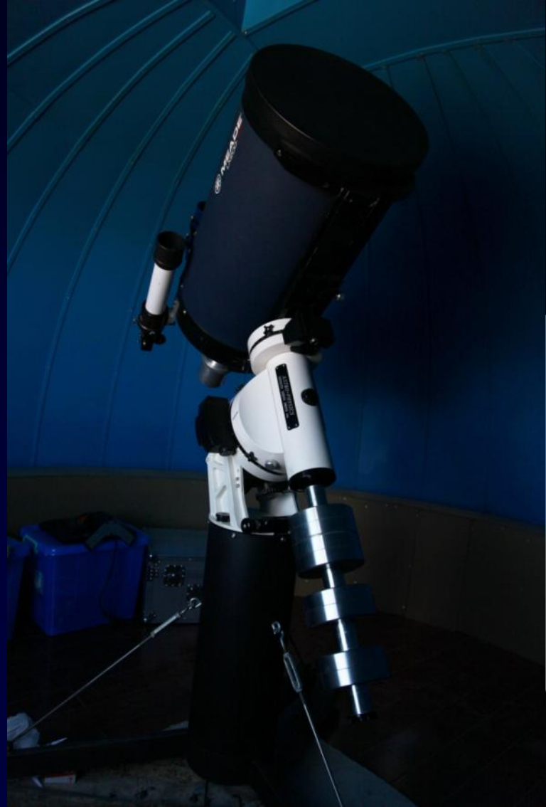
40cm Telescope for SCIDAR
